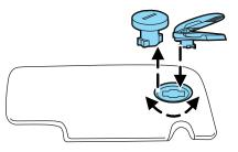
2. Insert the end of the storage accessory into the visor opening and turn 1/4-turn in either direction until the accessory snaps into place. For best results, ensure the open end of the accessory is facing away from the windshield.
